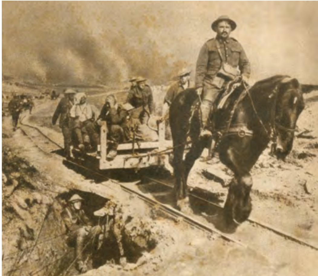
Wounded WWI Canadian soldiers on the way to rear dressing station. 1917. The horse-drawn narrow gauge rails were useful in the waterlogged battlefields of Flanders. Credit: Shutterstock, Everett Collection.
